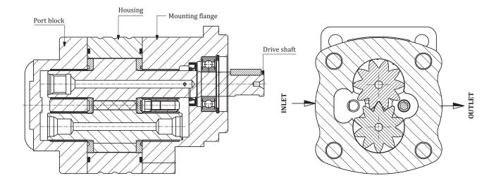
Long shaft journals (hydrodynamic bearing) provide superior bearing surface and premium material selection as well as the minimum number of rotating parts, contribute long efficient service life of VELJAN GEAR PUMPS.
