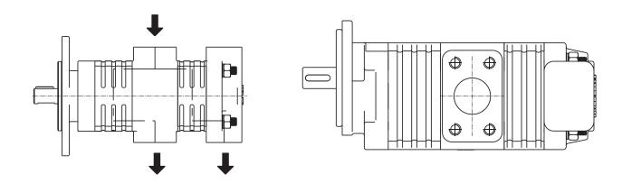
SEPERATED STAGES - B3 (Two Inlet , Two Outlets) - VGP - DB,DC
